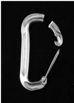
In test #2, all the sample carabiners broke at the small radius and exhibited substantial elongation. Test #3 samples all broke at the large radius – where the webbing was connected.
