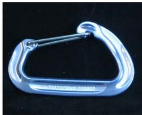
Carabiners were Black Diamond "Oz" wiregate "offset D" carabiners. These are smaller than would normally be used by most SAR teams, but have a low MBS of 20kN. We chose these to facilitate easier breaking.
