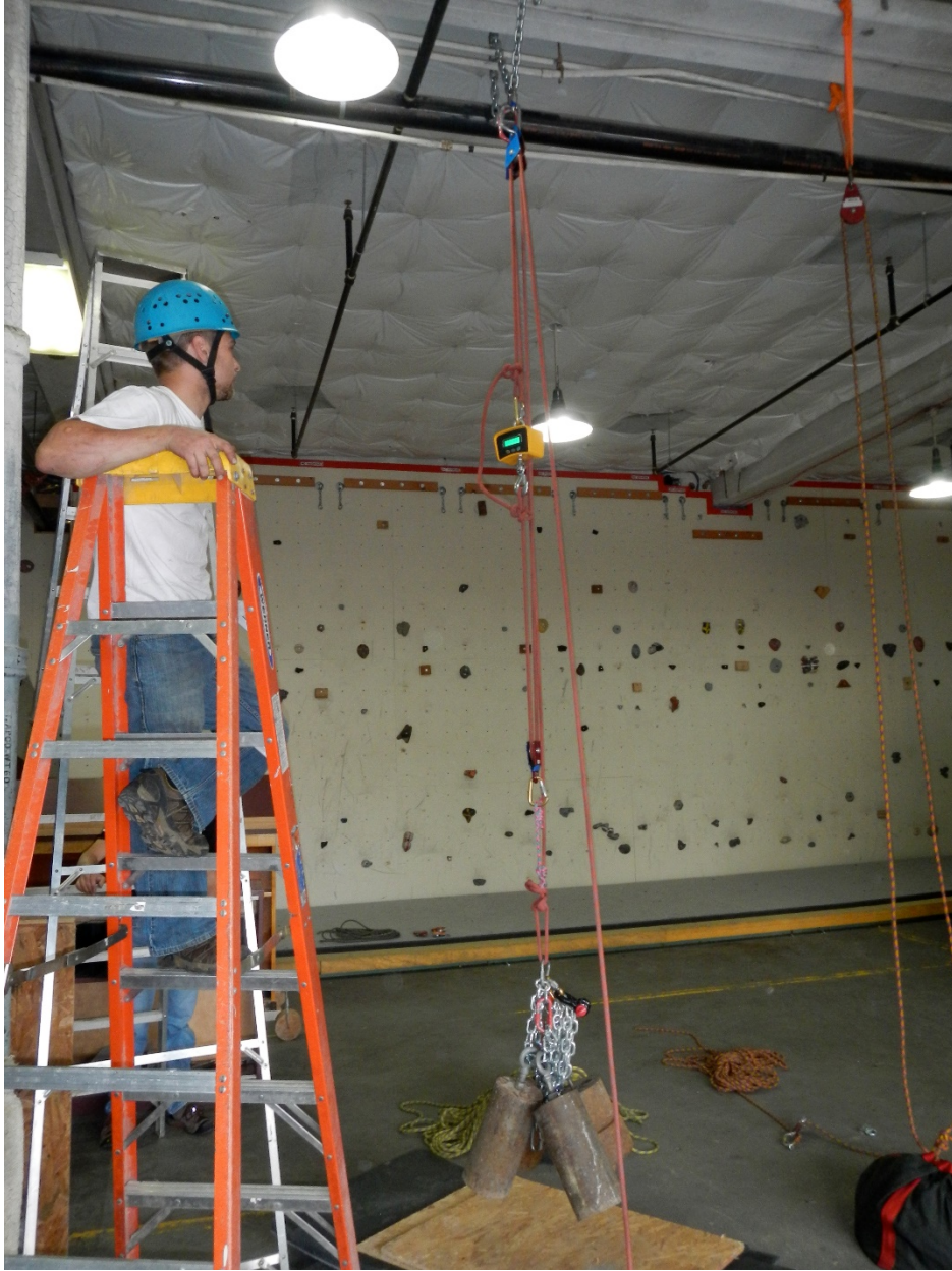
Figure 2. Photograph of 3-to-1 pulley raising test system.
