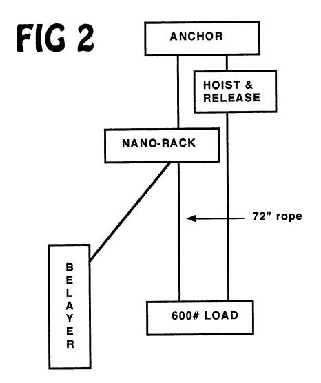
Initial test setup for determining belay competency of 3 bar Nano-Rack reeved in "belay configuration" using PMI 1/2" EZ Bend rope.
