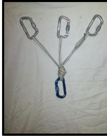
Three Leg Masterpoint – Mean Strength: 30kN
