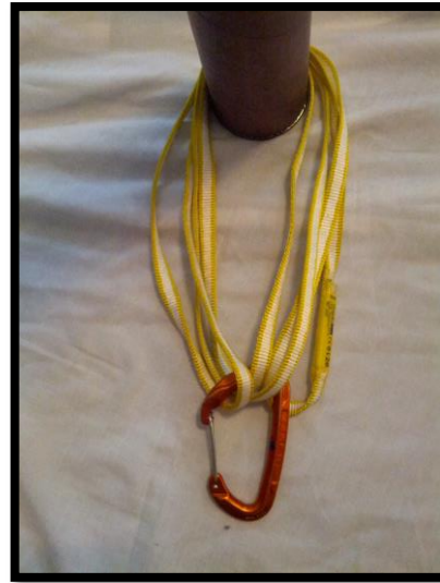
Wrap 2 Clip 4 – Mean Strength: 64kN
