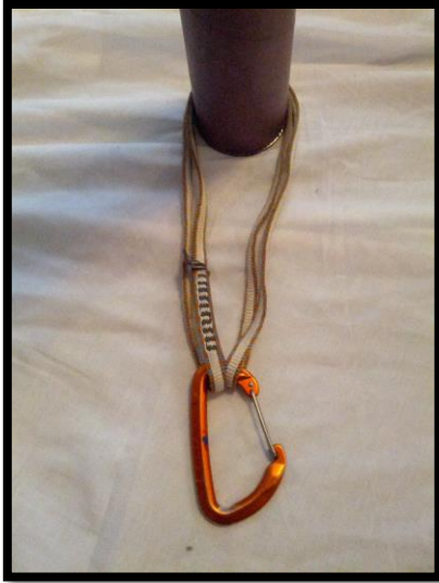
Basket Hitch – Mean Strength: 45 kN
