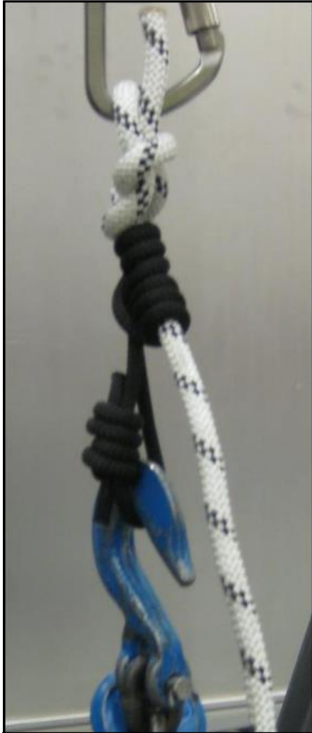
Figure 3: Pull test configuration. An SMC 45kN steel carabiner (1/4 inch bar stock), a bowline without a safety in 11 mm PMI EZ Bend rope, a three wrap prusik in 7 mm PMI accessory cord.
