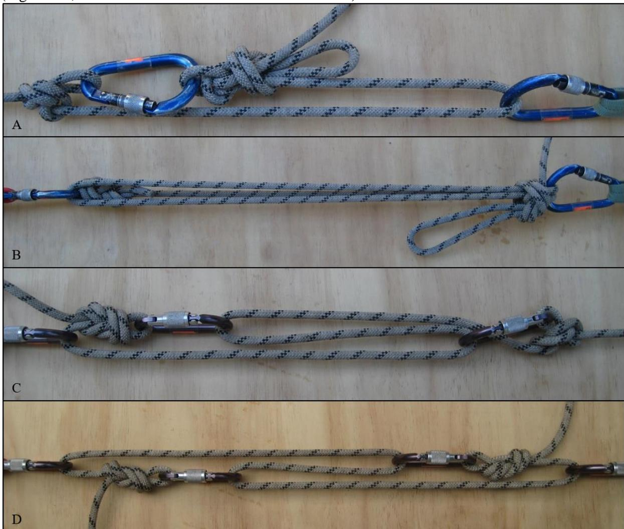
**Figure 1:** Examples of the four tensioning systems investigated. **A)** Trucker's Hitch locked off with a half hitch and an overhand on a bight, **B)** 3:1 Block and Tackle locked off with a half hitch and an overhand on a bight, **C)** Voodoo, **D)** Poldo. All these systems can be tied in a variety of configurations; only the variant tested is shown here. For additional examples of the Voodoo and Poldo and illustrated directions on how to tie them, see Evans 2015b.
