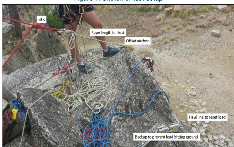
Figure 2: Actual test setup
