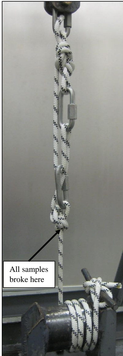
Figure 2: The Voodoo tensioning system built with a high strength tie off, butterfly, figure 8 on a bight, 11 mm PMI EZ Bend, and ½ inch hardware store screw links.
