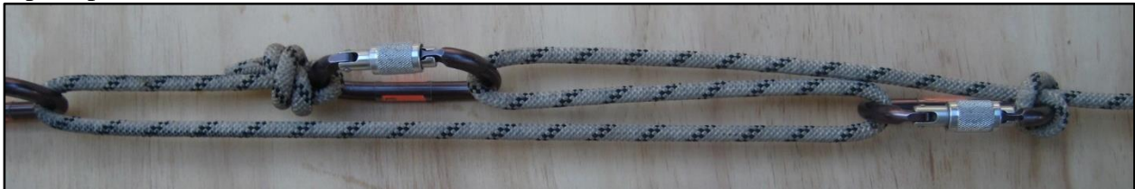
Figure 1: The Voodoo tensioning system constructed with a clove hitch and a slip barrel knot (Poacher's Knot in Ashley Book of Knots #409, p. 65). Many other configurations are possible (see Evans 2015 for more examples).
