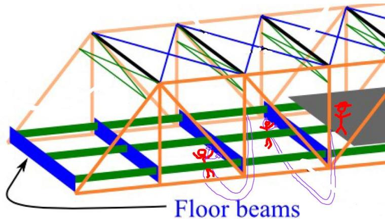
**Figure 1: Rope Access Floor beam Inspection Illustration**
