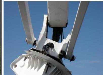
Photo 9: Snooper Truck Pin Failure.
