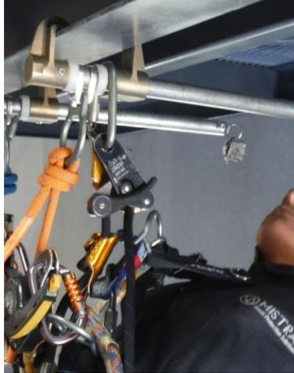
**Photo 14: Worker using beam clamps with releasable attachment (Grillon).**
