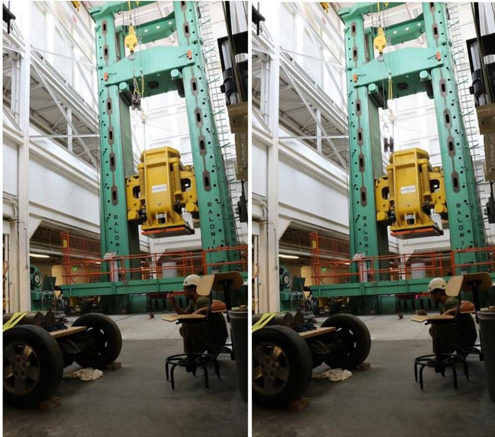
**Figure 6 – Drop Testing Setup: Pre-Drop (Left) and Post-Drop (Right)**
