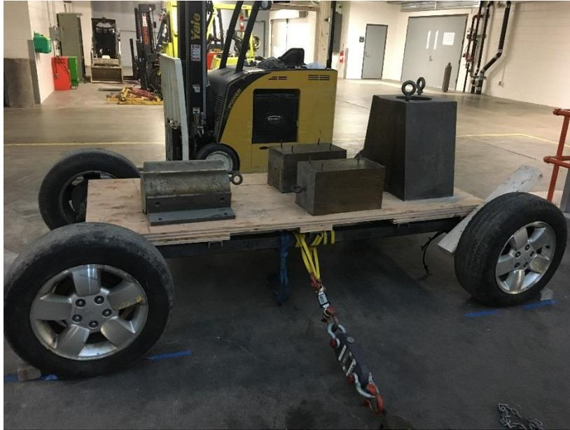
**Figure 2 – Test Vehicle Shown Fully Loaded (Test Setup #3) During Static Testing**
