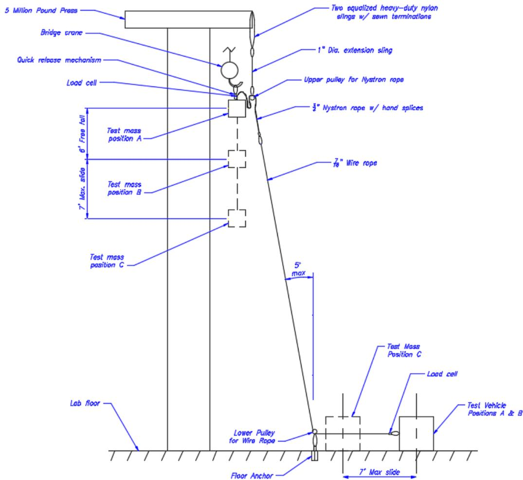
**Figure 1 - Drop Testing Schematic**
