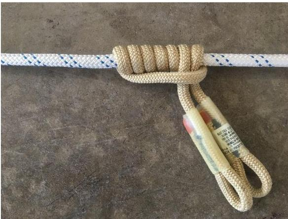
Figure 1. 6/1 Asymmetric VT Prusik on 11mm Rope
