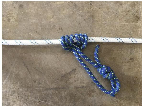
Figure 2. 3/3 Symmetric Prusik on 11mm Rope
